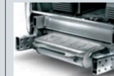
Two different interfaces for original Al-Ko AMC chassis, for ultimate quality coupling when the vehicle is supplied in the Tractor cab or Tractor chassis cowl version.
