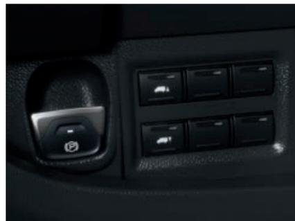
The electric park brake provides greater comfort in everyday usage. Driver can activate holding mechanism by a dedicated switch located on dashboard; functionality can even be automatically enabled through a specific instrument cluster setting.
