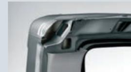
The cab, already set up for conversion (with reinforced cab pillars, without roof or rear partition), offers factory quality for all outfittings and Fiat Professional type-approval of the seat belts.
