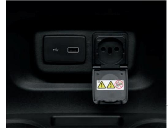
The 230v power socket helps to easily charge electric devices such as laptops, electric tool batteries, tablets, smartphones and other low power appliances that require electricity up to 150 Watts.
