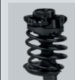
McPherson front suspension with independent wheels, standard front and rear anti-roll bar reinforced springs for motorhome versions. New higher front suspension available where necessary.
