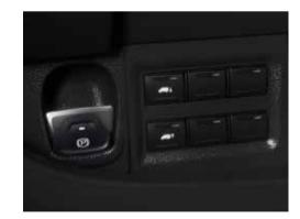
The new electric park brake provides greater comfort in everyday usage. Driver can activate holding mechanism by a dedicated switch located on dashboard; functionality can even be automatically enabled through a specific instrument
