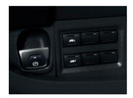
The electric park brake provides greater comfort in everyday usage. Driver can activate holding mechanism by a dedicated switch located on dashboard; functionality can even be automatically enabled through a specific instrument
